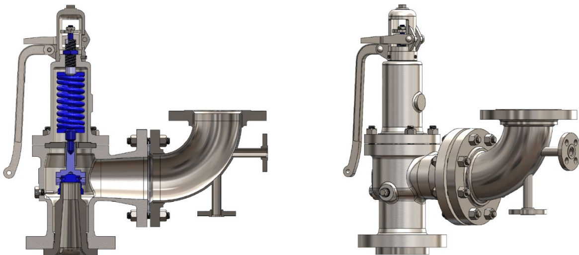
Figure 26. Small-diameter elbow water seal type
