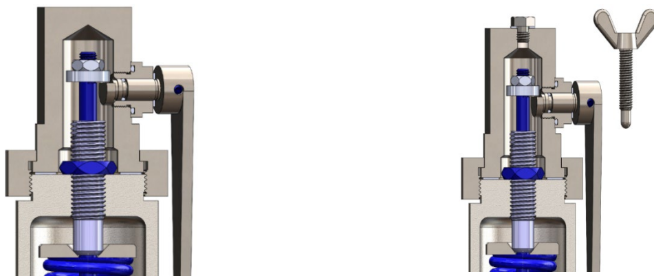
Figure 8. Bolted sealed lever cap
